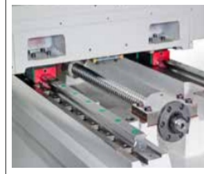
LINEAR GUIDE WAYS C3 40mm BALL SCREWS
