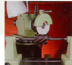
ATTACHMENT FOR SHARPENING HOBBS / AZDIRMA ÇAKISI BİLEME APARATI
