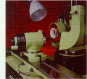
ATTACHMENT FOR GRINDING ROUGHING REAMERS / RAYBA BİLEME APARATI
